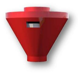
EQUIPMENT TRANSFERS THE REQUIRED CEMENT COMING FROM THE SILO WITH THE CEMENT SCREW TO THE MIXTURE IN THE MIXER. EQUIPMENT HAS 100 KG MEASURING CAPACITY. DISCHARGE PROVIDES BY PNEUMATIC VALVE. POSITIONED ON THE MIXER.LEVEL CONTROL MADE BY OPERATOR. START-STOP OPERATION MADE BY BUTTONS ON THE PANEL.TRANSFERS THE CEMENT TO THE MIXER WITH HELP OF PNEUMATIC VALVE. OPERATOR,PROVIDES DISCHARGE WITH THE PNEUMATIC JOISTIC.
