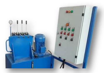
MACHINE ELECTRIC PANEL; OPERATING SYSTEM EXIST OF COLLECTED POWER AND CONTROL PANELS GATHERED IN ONE UNIT. DESIGNED TO OPERATION ORDER. THERE ARE STOP BUTTONS TO INTERVENE IN CASE OF EMERGENCY. USED MATERIALS ARE SCHNEIDER AND SIEMENS BRAND. INCLUDED PROTECTION INSURANCE FOR ALL MOTORS. USED SCHNEIDER BRAND TIMER FOR TIMING COMMANDS.
