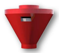
EQUIPMENT TRANSFERS THE REQUIRED CEMENT COMING FROM THE SILO WITH THE CEMENT SCREW TO THE MIXTURE IN THE MIXER. EQUIPMENT HAS 100 KG MEASURING CAPACITY. DISCHARGE PROVIDES BY PNEUMATIC VALVE. POSITIONED ON THE MIXER.LEVEL CONTROL MADE BY OPERATOR. START-STOP OPERATION MADE BY BUTTONS ON THE PANEL.TRANSFERS THE CEMENT TO THE MIXER WITH HELP OF PNEUMATIC VALVE. OPERATOR, PROVIDES DISCHARGE WITH THE PNEUMATIC JOISTIC.
