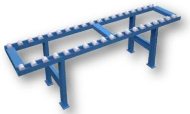
POSITIONED TO END OF THE MACHINE. TAKES THE FULL PALLET TO THE MANUAL PALLET CARRIER. PALLETS PUSH EACH OTHER. WITH THIS CONVEYOR OPERATOR SAVE THE TIME. USING IT WITHOUT ENERGY WITH ROLLER SYSTEM ON IT. MANUAL PALLET CARRIER HELPS PALLETS TAKE FROM THE CONVEYOR TO THE DRYING AREA.
