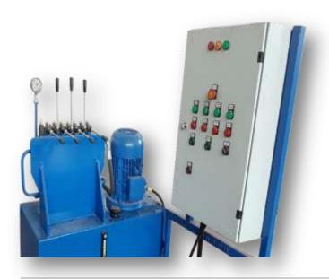
MACHINE OPERATOR PLATFORM; OPERATOR OBSERVE THE MACHINE AND ALL MOVEMENTS ARE PROVIDED VIA HYDRAULIC CONTROL HANDLE AND IS EASY TO USE.
