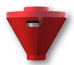
EQUIPMENT TRANSFERS THE REQUIRED CEMENT COMING FROM THE SILO WITH THE CEMENT SCREW TO THE MIXTURE IN THE MIXER. EQUIPMENT HAS 50 KG MEASURING CAPACITY. DISCHARGE PROVIDES BY PNEUMATIC VALVE. POSITIONED ON THE MIXER.LEVEL CONTROL MADE BY OPERATOR. START-STOP OPERATION MADE BY BUTTONS ON THE PANEL.TRANSFERS THE CEMENT TO THE MIXER WITH HELP OF PNEUMATIC VALVE. OPERATOR, PROVIDES DISCHARGE WITH THE PNEUMATIC JOISTIC.
