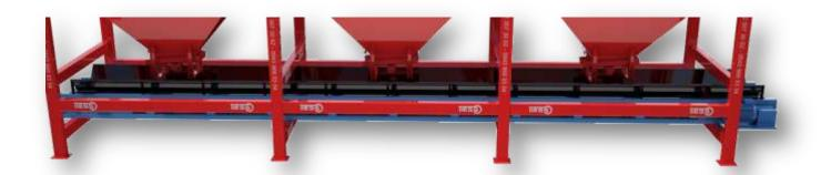
THIS CONVEYOR ALLOWS THE WEIGHING OF THE AGGREGATE IN THE HOPPER AND AFTER WEIGHING TRANSFERS THE AGGREGATE TO THE TRANSFER BAND. POSITIONED JUST BELOW THE AGGREGA HOPPER. MAIN CHASSIS IS MANUFACTURED TO THE NORMS OF ISO 9001 QUALITY AND TO THE DIN NORMS, USING 40 x 80 x 3mm Profile and 3mm. Sheet Metal. Roll Stations are placed each 90 cm to prevent the Flee Back. The Rubber Band is made with 8 mm cord material. Rolls are 3"(ø 89 mm ). Driven by Reducer Group. Motor power is 2,2 kw.
