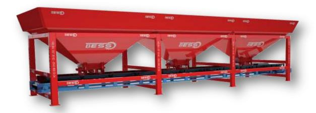
THIS HOPPER IS THE EQUIPMENT FOR MATERIALS AS SAND, GRAVEL, STONE DUST ETC. NEEDED FOR THE MIXTURE. UNDER EACH HOPPER ARE 1 UNLOADING COVERS. **CHASSIS** IS MANUFACTURED TO THE NORMS OF ISO 9001 QUALITY AND ACCORDING TO ALL DIN NORMS USING 150 x 100 x 6 mm. THICK PROFILE AND METAL SHEET. THICK METAL SHEET IS USED. METAL SHEET. THE FLOWING IS STRENGTHENED WITH THE VIBROMOTOR ON THE HOPPER.
