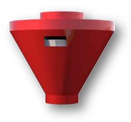
EQUIPMENT TRANSFERS THE REQUIRED CEMENT COMING FROM THE SILO WITH THE CEMENT SCREW TO THE MIXTURE IN THE MIXER. EQUIPMENT HAS 50 KG MEASURING CAPACITY. DISCHARGE PROVIDES BY PNEUMATIC VALVE. POSITIONED ON THE MIXER.LEVEL CONTROL MADE BY OPERATOR. START-STOP OPERATION MADE BY BUTTONS ON THE PANEL.TRANSFERS THE CEMENT TO THE MIXER WITH HELP OF PNEUMATIC VALVE. OPERATOR,PROVIDES DISCHARGE WITH THE PNEUMATIC JOISTIC.
