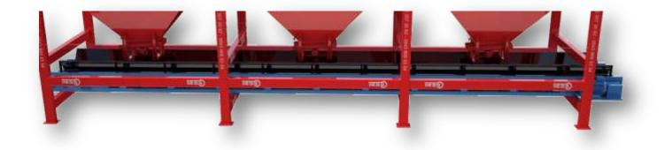
THIS CONVEYOR ALLOWS THE WEIGHING OF THE AGGREGATE IN THE HOPPER AND AFTER WEIGHING TRANSFERS THE AGGREGATE TO THE TRANSFER BAND. POSITIONED JUST BELOW THE AGGREGA HOPPER. MAIN CHASSIS IS MANUFACTURED TO THE NORMS OF ISO 9001 QUALITY AND TO THE DIN NORMS, USING 40 x 80 x 3mm PROFILE AND 3mm. SHEET METAL. ROLL STATIONS ARE PLACED EACH 90 cm TO PREVENT THE FLEE BACK. THE RUBBER BAND IS MADE WITH 8 mm CORD MATERIAL. ROLLS ARE 3"(Ø 89 mm). DRIVEN BY REDUCER GROUP. MOTOR POWER IS 2,2 kw.
