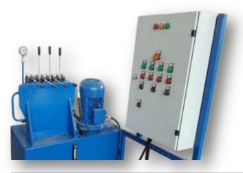
MACHINE OPERATOR PLATFORM; OPERATOR OBSERVE THE MACHINE AND ALL MOVEMENTS ARE PROVIDED VIA HYDRAULIC CONTROL HANDLE AND IS EASY TO USE.
