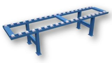
POSITIONED TO END OF THE MACHINE. TAKES THE FULL PALLET TO THE MANUAL PALLET CARRIER. PALLETS PUSH EACH OTHER. WITH THIS CONVEYOR OPERATOR SAVE THE TIME. USING IT WITHOUT ENERGY WITH ROLLER SYSTEM ON IT. MANUAL PALLET CARRIER HELPS PALLETS TAKE FROM THE CONVEYOR TO THE DRYING AREA.
