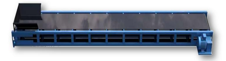
EQUIPMENT IS POSITIONED ON THE OUTPUT OF THE MIXER. TRANSFERS THE PREPARED MORTAR TO THE MORTAR HOPPER. THE MAIN CHASSIS IS MANUFACTURED TO THE NORMS OF ISO 9001 QUALITY USING 40 x 80 x 3mm PROFILE AND 3mm. SHEET METAL. THERE IS A SHEET METAL THAT PREVENTS ESCAPING BACK OF THE MATERIALS OF THE BAND. THE BAND RUBBERS ARE MANUFACTURED WITH 4 LAYERS FROM 8 mm. CORD MATERIAL. ROLLS ARE 3'(Ø 60mm). ROLLS POSITIONS ARE PLACED 1 BY EACH 90 cm. DRIVEN BY MOTOR AND REDUCER GROUP.MOTOR POWER IS 2,2 kw.
