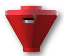
EQUIPMENT TRANSFERS THE REQUIRED CEMENT COMING FROM THE SILO WITH THE CEMENT SCREW TO THE MIXTURE IN THE MIXER. EQUIPMENT HAS 100 KG MEASURING CAPACITY. DISCHARGE PROVIDES BY PNEUMATIC VALVE. POSITIONED ON THE MIXER.LEVEL CONTROL MADE BY OPERATOR. START-STOP OPERATION MADE BY BUTTONS ON THE PANEL.TRANSFERS THE CEMENT TO THE MIXER WITH HELP OF PNEUMATIC VALVE. OPERATOR, PROVIDES DISCHARGE WITH THE PNEUMATIC JOISTIC.
