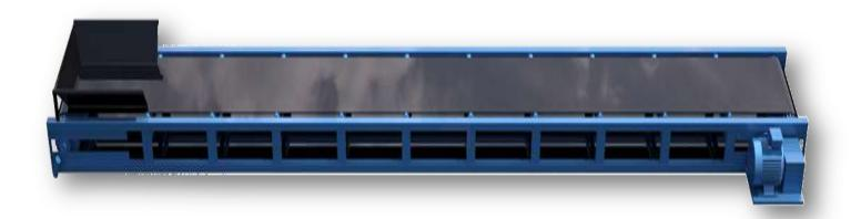
EQUIPMENT IS POSITIONED ON THE OUTPUT OF THE MIXER. TRANSFERS THE PREPARED MORTAR TO THE MORTAR HOPPER. THE MAIN CHASSIS IS MANUFACTURED TO THE NORMS OF ISO 9001 QUALITY USING 40 x 80 x 3mm PROFILE AND 3mm. SHEET METAL. THERE IS A SHEET METAL THAT PREVENTS ESCAPING BACK OF THE MATERIALS OF THE BAND. THE BAND RUBBERS ARE MANUFACTURED WITH 4 LAYERS FROM 8 mm. CORD MATERIAL. ROLLS ARE 3'(Ø 60mm). ROLLS POSITIONS ARE PLACED 1 BY EACH 90 cm. DRIVEN BY MOTOR AND REDUCER GROUP.MOTOR POWER IS 2,2 kw.
