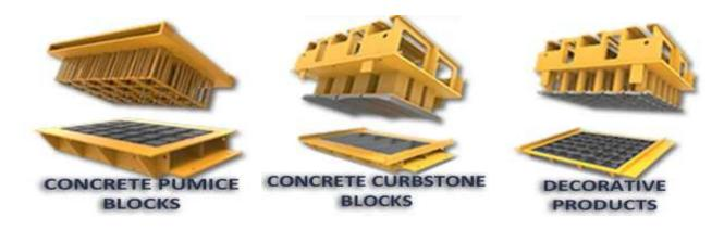
PAVING BLOCK MOULD MONOBLOCK: MANUFACTURED FROM SPECIAL MOULD STEEL. PRESSING LININGS ARE TO BE ACCUSTOMED IN TO THE MOULD SECTION. IS READY TO USE AFTER HARDENING WITH INDUCTION. STEEL CONSTRUCTION MOULDS: AFTER DESIGNING THE MOULDS DIMENSIONS WILL BE BROUGHT TO THE DESIRED VALUE USING WEAR RESISTANT SPECIAL SHEET METAL WITH STEEL CONSTRUCTION SYSTEM. CURBSTONE MOULD BLADES ARE READY TO USE AFTER SAWDUST REMOVAL PROCESSING FROM THE CK 45 SHEET METALS AND HARDENINGS PROCESS VIA INDUCTION.
