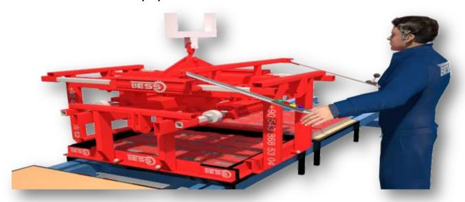
CURED AND DRIED PRODUCTS COMING FROM REAR UNLOADER ROBOT, TAKEN FROM THE PALLETS WITH OPERATOR CONTROL AND STACKED ON EURO SHIPPING PALLETS. MOVES WITH PNEUMATIC SYSTEM. PROVIDES ITS COLLECTING OPERATION QUICKLY AT ONE POINT. WITH MOTOR ON IT, MOVES RIGHT-LEFT AND UP-DOWN. MOTOR POWER IS 0,2 KW.
