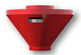
EQUIPMENT TRANSFERS THE REQUIRED CEMENT COMING FROM THE SILO WITH THE CEMENT SCREW TO THE MIXTURE IN THE MIXER. EQUIPMENT HAS 50 KG MEASURING CAPACITY. DISCHARGE PROVIDES BY PNEUMATIC VALVE. POSITIONED ON THE MIXER.LEVEL CONTROL MADE BY OPERATOR. START-STOP OPERATION MADE BY BUTTONS ON THE PANEL.CEMENT MEASURING MADE BY GLASS LEVEL INDICATOR. OPERATOR, PROVIDES DISCHARGE WITH THE PNEUMATIC JOISTIC.
