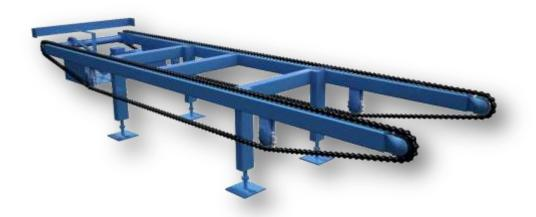
IT IS THE LIFTING SYSTEM FOR THE PRODUCTS PRESSED BY THE MACHINE ON THE PALLETS TO THE FRONT FULL STACKING ROBOT. WORKS WITH THE HELP OF MOTOR WITH REDUCTOR AND CHAIN GEAR. START-STOP ITSELF ACCORDING TO COMMAND FROM THE SWITCH ON IT. ENGINE POWER IS 2.2 KW.
