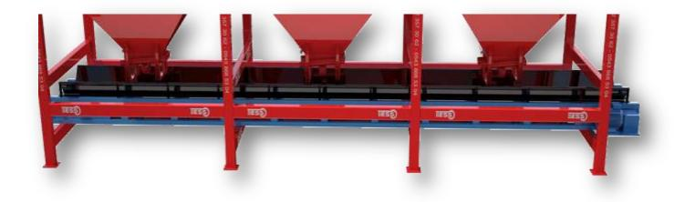
THIS CONVEYOR ALLOWS THE WEIGHING OF THE AGGREGATE IN THE HOPPER AND AFTER WEIGHING TRANSFERS THE AGGREGATE TO THE TRANSFER BAND. POSITIONED JUST BELOW THE AGGREGA HOPPER. MAIN CHASSIS IS MANUFACTURED TO THE NORMS OF ISO 9001 QUALITY AND TO THE DIN NORMS, USING 40 x 80 x 3mm PROFILE AND 3mm. SHEET METAL. ROLL STATIONS ARE PLACED EACH 90 cm TO PREVENT THE FLEE BACK. THE RUBBER BAND IS MADE WITH 8 mm CORD MATERIAL. ROLLS ARE 3''(Ø 89 mm ). DRIVEN BY REDUCER GROUP. MOTOR POWER IS 2,2 kw.
