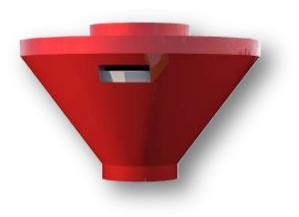
EQUIPMENT TRANSFERS THE REQUIRED CEMENT COMING FROM THE SILO WITH THE CEMENT SCREW TO THE MIXTURE IN THE MIXER. EQUIPMENT HAS 50 KG MEASURING CAPACITY. DISCHARGE PROVIDES BY PNEUMATIC VALVE. POSITIONED ON THE MIXER.LEVEL CONTROL MADE BY OPERATOR. START-STOP OPERATION MADE BY BUTTONS ON THE PANEL.CEMENT MEASURING MADE BY GLASS LEVEL INDICATOR. OPERATOR,PROVIDES DISCHARGE WITH THE PNEUMATIC JOISTIC.
