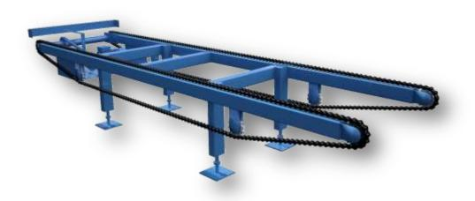
IT IS THE LIFTING SYSTEM FOR THE PRODUCTS PRESSED BY THE MACHINE ON THE PALLETS TO THE FRONT FULL STACKING ROBOT. WORKS WITH THE HELP OF MOTOR WITH REDUCTOR AND CHAIN GEAR. START-STOP ITSELF ACCORDING TO COMMAND FROM THE SWITCH ON IT. ENGINE POWER IS 2.2 KW.
