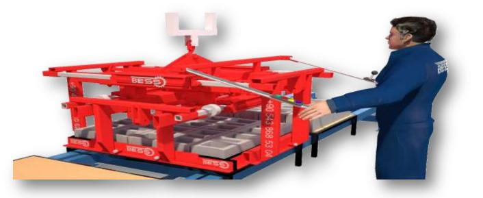
CURED AND DRIED PRODUCTS COMING FROM REAR UNLOADER ROBOT, TAKEN FROM THE PALLETS WITH OPERATOR CONTROL AND STACKED ON EURO SHIPPING PALLETS. MOVES WITH PNEUMATIC SYSTEM. PROVIDES ITS COLLECTING OPERATION QUICKLY AT ONE POINT. WITH MOTOR ON IT, MOVES RIGHT-LEFT AND UP-DOWN. MOTOR POWER IS 0,2 KW.
