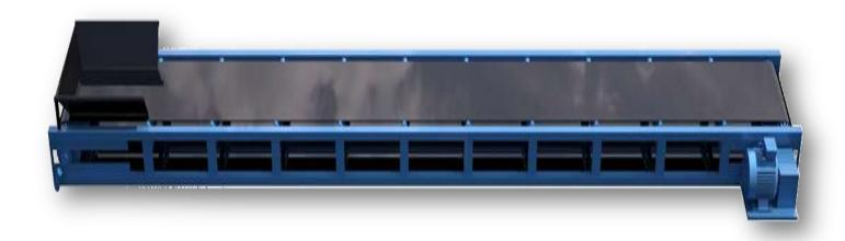
EQUIPMENT IS POSITIONED ON THE OUTPUT OF THE MIXER. TRANSFERS THE PREPARED MORTAR TO THE MORTAR HOPPER. THE MAIN CHASSIS IS MANUFACTURED TO THE NORMS OF ISO 9001 QUALITY USING 40 x 80 x 3mm PROFILE AND 3mm. SHEET METAL. THERE IS A SHEET METAL THAT PREVENTS ESCAPING BACK OF THE MATERIALS OF THE BAND. THE BAND RUBBERS ARE MANUFACTURED WITH 4 LAYERS FROM 8 mm. CORD MATERIAL. ROLLS ARE 3'(ø 60mm). ROLLS POSITIONS ARE PLACED 1 BY EACH 90 cm. DRIVEN BY MOTOR AND REDUCER GROUP.MOTOR POWER IS 2,2 kw.
