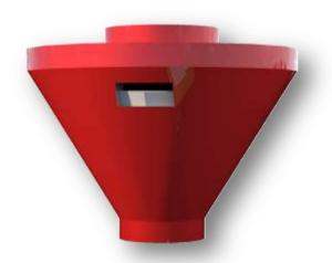
EQUIPMENT TRANSFERS THE REQUIRED CEMENT COMING FROM THE SILO WITH THE CEMENT SCREW TO THE MIXTURE IN THE MIXER. EQUIPMENT HAS 100 KG MEASURING CAPACITY. DISCHARGE PROVIDES BY PNEUMATIC VALVE. POSITIONED ON THE MIXER.LEVEL CONTROL MADE BY OPERATOR. START-STOP OPERATION MADE BY BUTTONS ON THE PANEL.CEMENT MEASURING MADE BY GLASS LEVEL INDICATOR. OPERATOR, PROVIDES DISCHARGE WITH THE PNEUMATIC JOISTIC.
