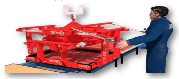
CURED AND DRIED PRODUCTS COMING FROM REAR UNLOADER ROBOT, TAKEN FROM THE PALLETS WITH OPERATOR CONTROL AND STACKED ON EURO SHIPPING PALLETS. MOVES WITH PNEUMATIC SYSTEM. PROVIDES ITS COLLECTING OPERATION QUICKLY AT ONE POINT. WITH MOTOR ON IT, MOVES RIGHT-LEFT AND UP-DOWN. MOTOR POWER IS 0,2 KW.
