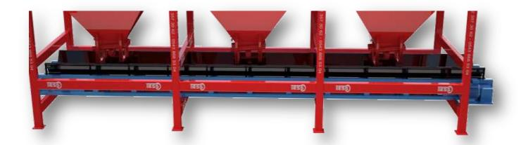
THIS CONVEYOR ALLOWS THE WEIGHING OF THE AGGREGATE IN THE HOPPER AND AFTER WEIGHING TRANSFERS THE AGGREGATE TO THE TRANSFER BAND. POSITIONED JUST BELOW THE AGGREGA HOPPER. MAIN CHASSIS IS MANUFACTURED TO THE NORMS OF ISO 9001 QUALITY AND TO THE DIN NORMS, USING 40 x 80 x 3mm PROFILE AND 3mm. SHEET METAL. ROLL STATIONS ARE PLACED EACH 90 cm TO PREVENT THE FLEE BACK. THE RUBBER BAND IS MADE WITH 8 mm CORD MATERIAL. ROLLS ARE 3"(\$\phi\$ 89 mm ). DRIVEN BY REDUCER GROUP. MOTOR POWER IS 2,2 kw.
