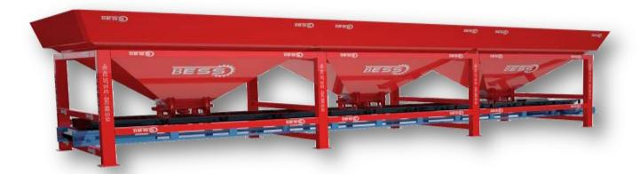
THIS HOPPER IS THE EQUIPMENT FOR MATERIALS AS SAND, GRAVEL, STONE DUST ETC. NEEDED FOR THE MIXTURE. UNDER EACH HOPPER ARE 1 UNLOADING COVERS. **CHASSIS** IS MANUFACTURED TO THE NORMS OF ISO 9001 QUALITY AND ACCORDING TO ALL DIN NORMS USING 150 x 100 x 6 mm. THICK PROFILE AND METAL SHEET. THICK METAL SHEET IS USED. METAL SHEET, THE FLOWING IS STRENGTHENED WITH THE VIBROMOTOR ON THE HOPPER.
